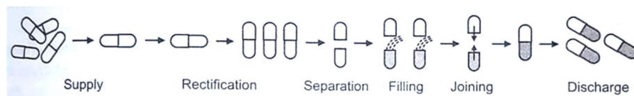
Fig. 5.5: Process of filling hard gelatin capsule
